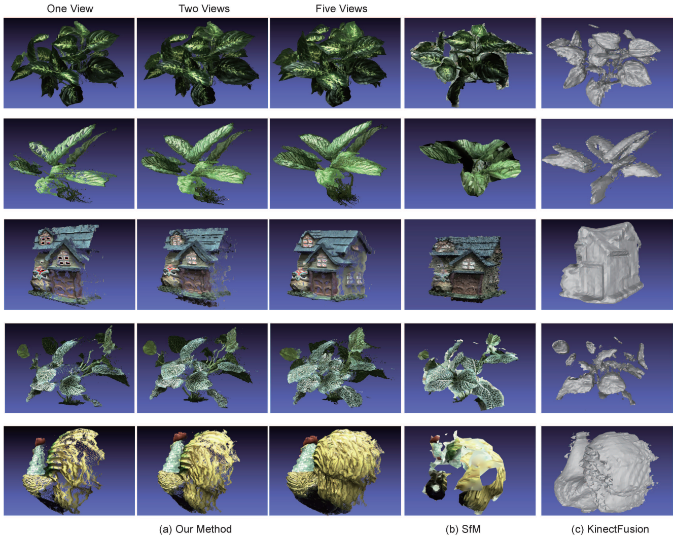
Figure 7. Our results vs. SfM and Kinect. For each model, we illustrate our reconstruction result using 1 view (i.e., the disparity map), 2 views, and 5 views. We also compare with the results generated using SfM and Kinect.
